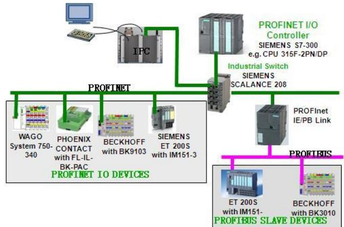
Figure 8. Architecture of PROFINET on SIEMENS Platform.
