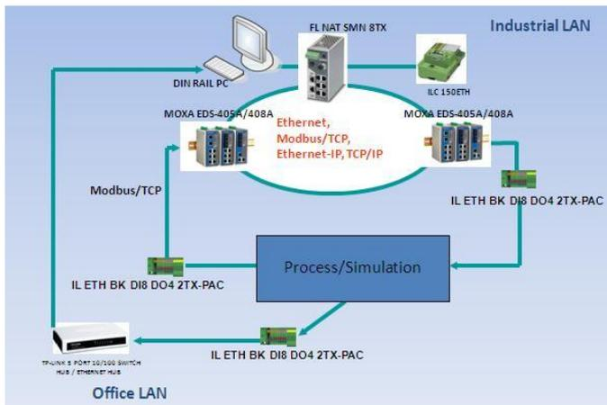
Figure 7. Structure for Ethernet based I/O systems module.
