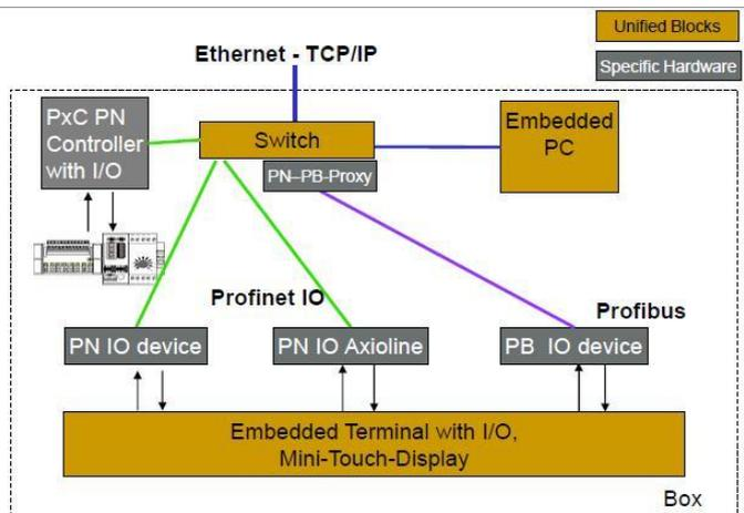
Figure 9. Architecture of Profinet on Phoenix Contact Platform.
