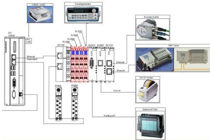
Figure 10. EtherCAT configuration.
