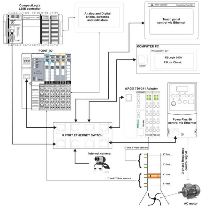
Figure 11. Ethernet IP laboratory setup.
