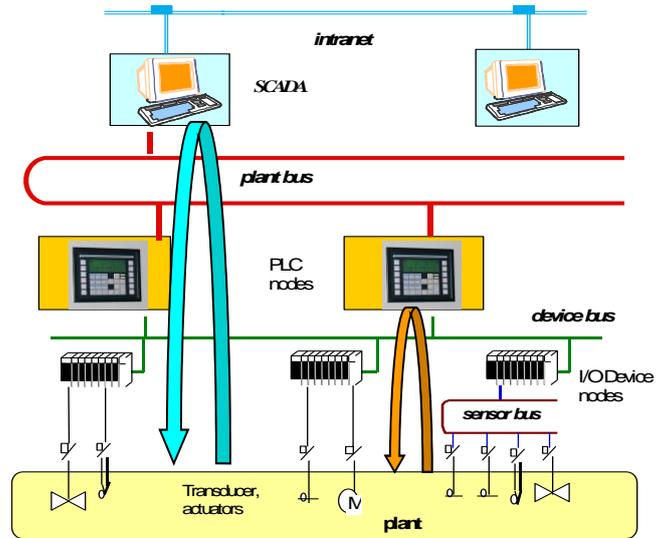
Figure 2. Multilevel structure of the industrial automation system
