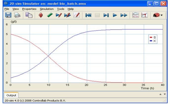
Figure 5. Time profiles of concentrations in the case of the batch prototype bioprocess.
