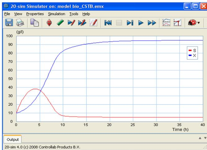
Figure 6. Evolution of concentrations - the continuous prototype bioprocess.
