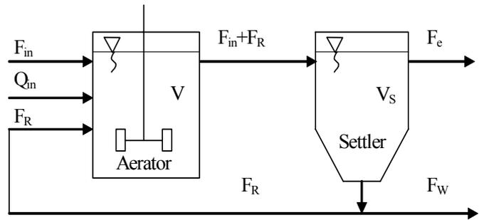
Figure 3. Schema of the activated sludge bioprocess.
